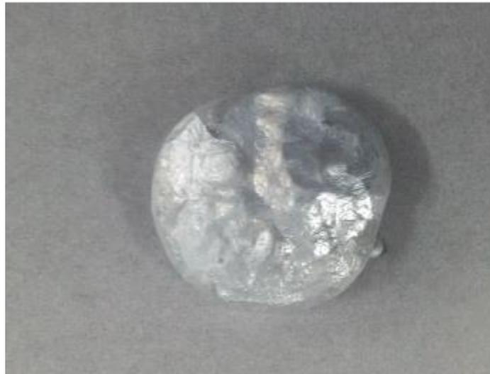
FIG. 7 High purity metallic zinc obtained by electrolysis
